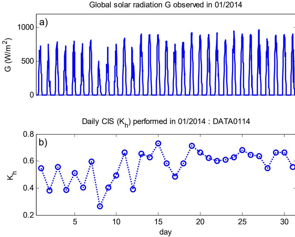
Fig. 2: Global solar radiation and Daily CIS performed in 01/2014, Can Tho city
